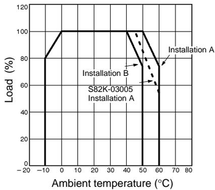
Note: When using the 7.5-W single-output models within the input voltage range between 90 and 110 VDC, the load rate will become 90% or less.
