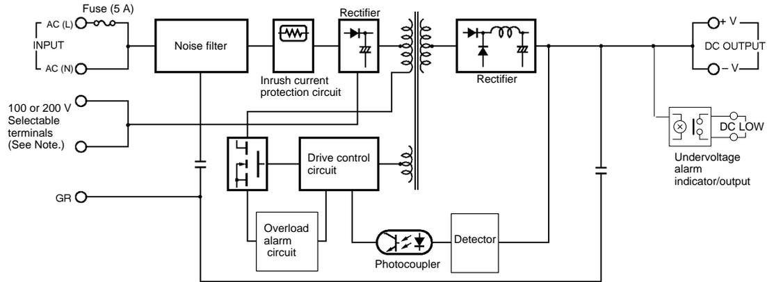
Note: Use the short bar to short-circuit terminals 7 and 8 to select 100 to 120 VAC and remove the short bar to select 200 to 240 VAC.
