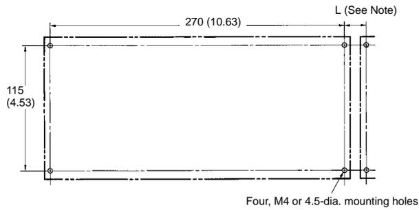
Note: If more than one Power Supply is installed in a row, keep a distance of 20 mm min. (L = 20 mm min.) between each adjacent Power Supply.
