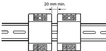
To mount the Power Supply on a DIN rail, hook portion (A) of the Power Supply to the rail and press the Power Supply toward direction (B).
