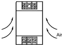
When mounting two or more Power Supplies side-by-side, allow at least 20 mm (0.79 in) spacing between them, as shown in the following illustration.
