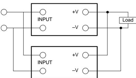
Note: When operating the 240-W model in parallel operation, set the switch to "PARALLEL." Refer to the derating curve for the rated current under this operation.
