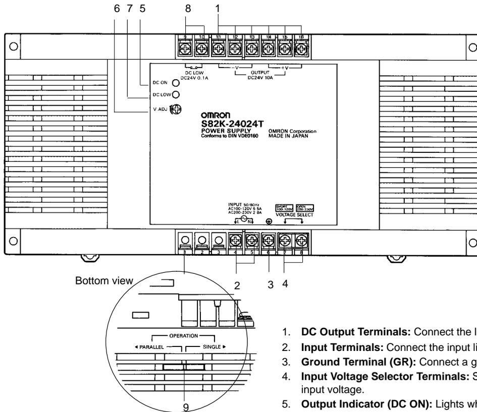
1. **DC Output Terminals:** Connect the load lines to these terminals.
