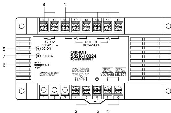
1. **DC Output Terminals:** Connect the load lines to these terminals.
