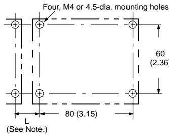
Note: If more than one Power Supply is installed in a row, keep a distance of 20 mm min. (L = 20 mm min.) between each adjacent Power Supply.
